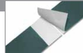
This method is good for two or more ply belts. The plies are separated carefully using a special equipment. Since the pressing process is made without using an adhesive compound, the joint area preserves the flexibility and the strength.
